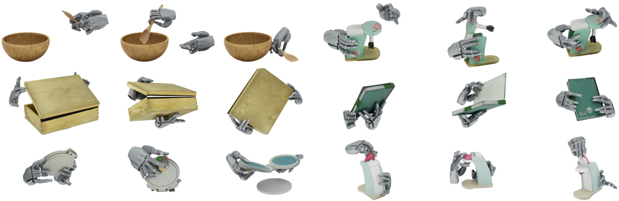
Figure 4: Contact Rich Tasks: The learned policies handle complex object interactions including picking, placing, handing over, stirring a bowl, and using articulations across objects of varying geometry.
